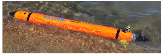
(b) The Riptide is torpedo-shaped AUV with 3 fins and one thruster as the back
